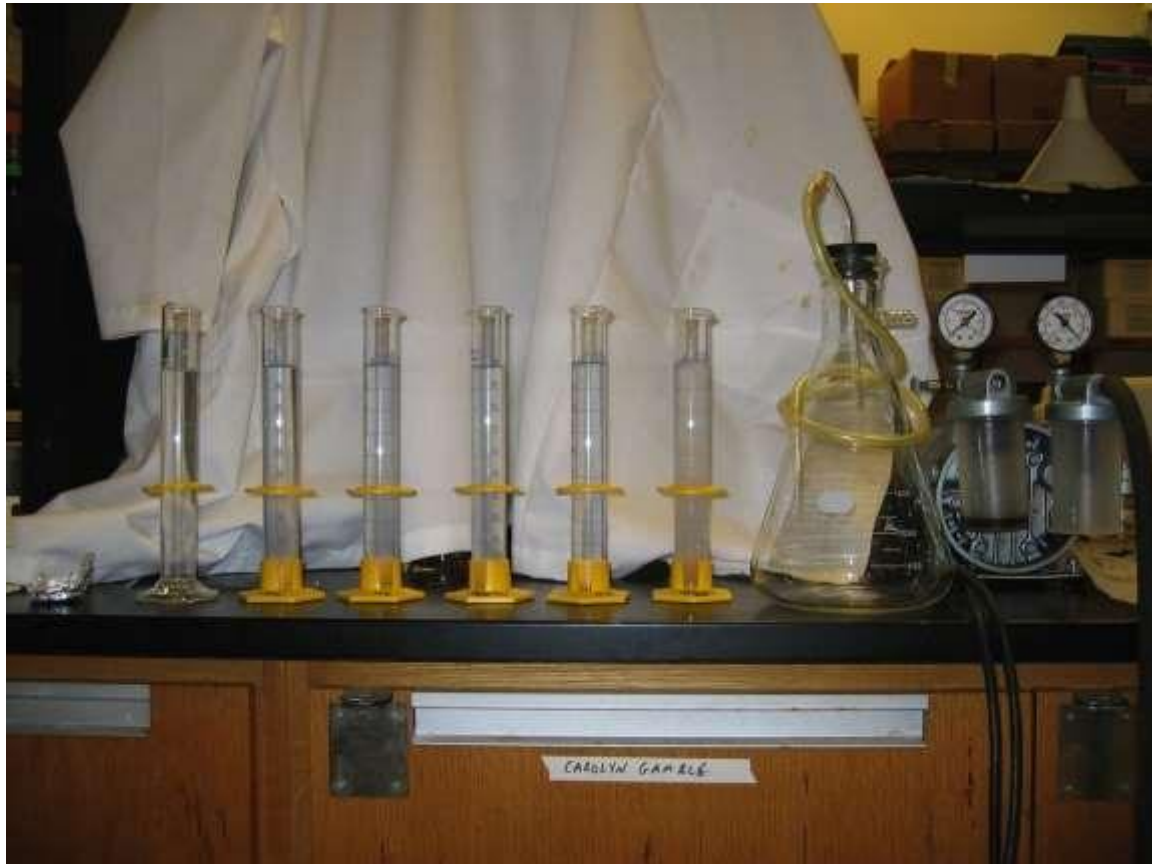
Figure 4. Suggested set up for gravity settling steps
