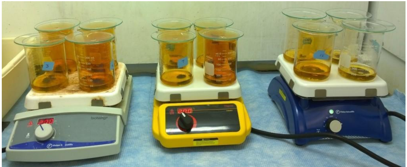
Figures 1 -2. Hotplate and glass beaker setup for acid digestion (hydrochloric and nitric acid treatment)
