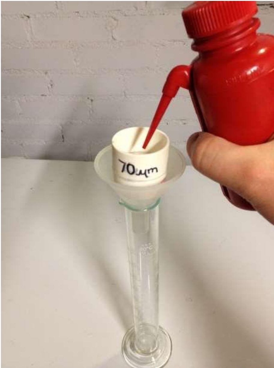
Figure 3. Small diameter sieve on graduated cylinder set up
