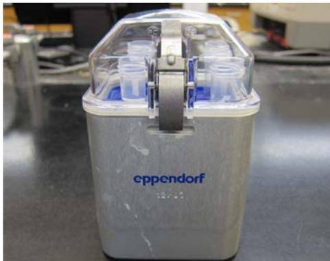
Fig. 1: Centrifuge bucket with vapor cap.
