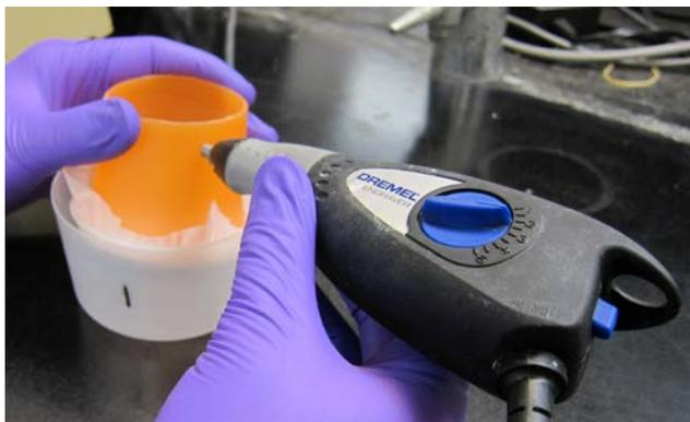
Fig. 25: How to use the electric engraver with the 7  $\mu$ m fabric.
