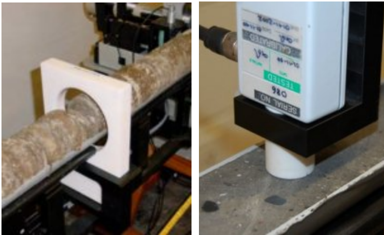
Figure 1. Loop (left) and point (right) sensors, mounted on core loggers (photos from http://www.geotek.co.uk ).
