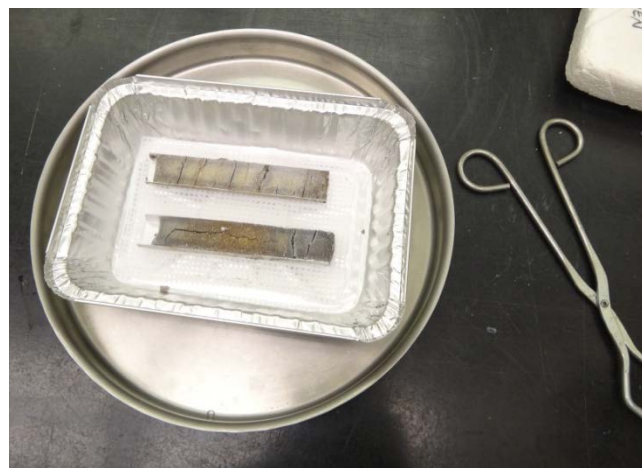
Figure 2. The two slab samples are completely frozen and placed in a metal freeze dryer tray for immediate freeze dry or storage in a freezer.
