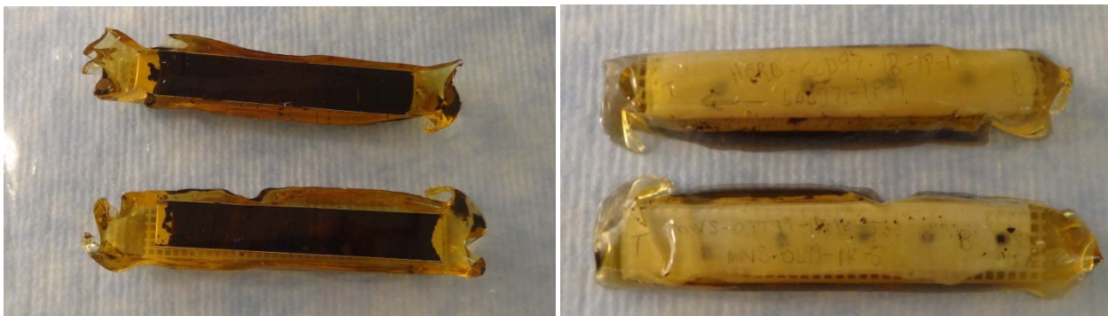
Figure 9. (Left) Finished product (top) Figure 10. (Right) finished product (bottom). Note the paper indicating which side of the sample is at the top (T) and bottom (B) of the core.
