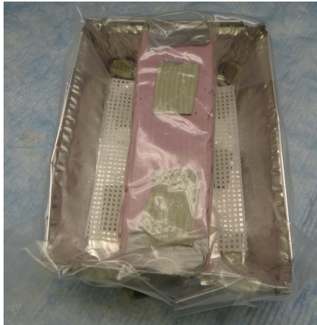
Figure 3. Metal tray set up for two thin sections: Pink insulation in the middle, covered by lay flat plastic tubing. Pieces of plastic craft mesh are cut to the appropriate size to cover the spaces where the thin sections will be placed.
