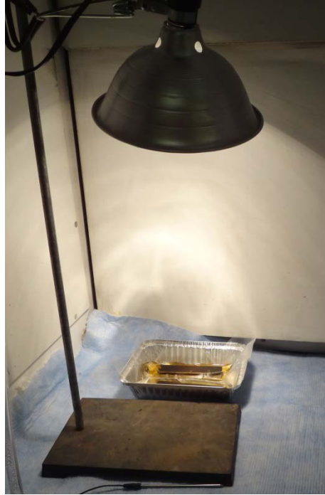
Figure 8. Epoxy cores curing via heat lamp in a fume hood. Note the heat lamp is approximately 45 cm above the cores so as not risk boiling the epoxy.
