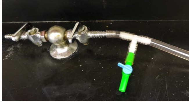
Figure 7. Vacuum set up (2). Note the use of the green T-switch, which allows for the vacuum to be broken without disconnecting the tubing.
