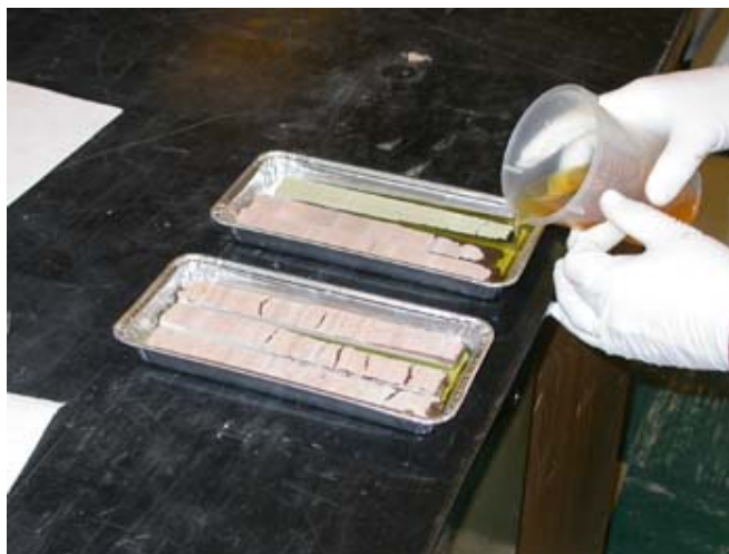
Adding resin. This can also be done while trays are in desiccator, and should be done under a hood. (figure courtesy of Pierre Francus)
