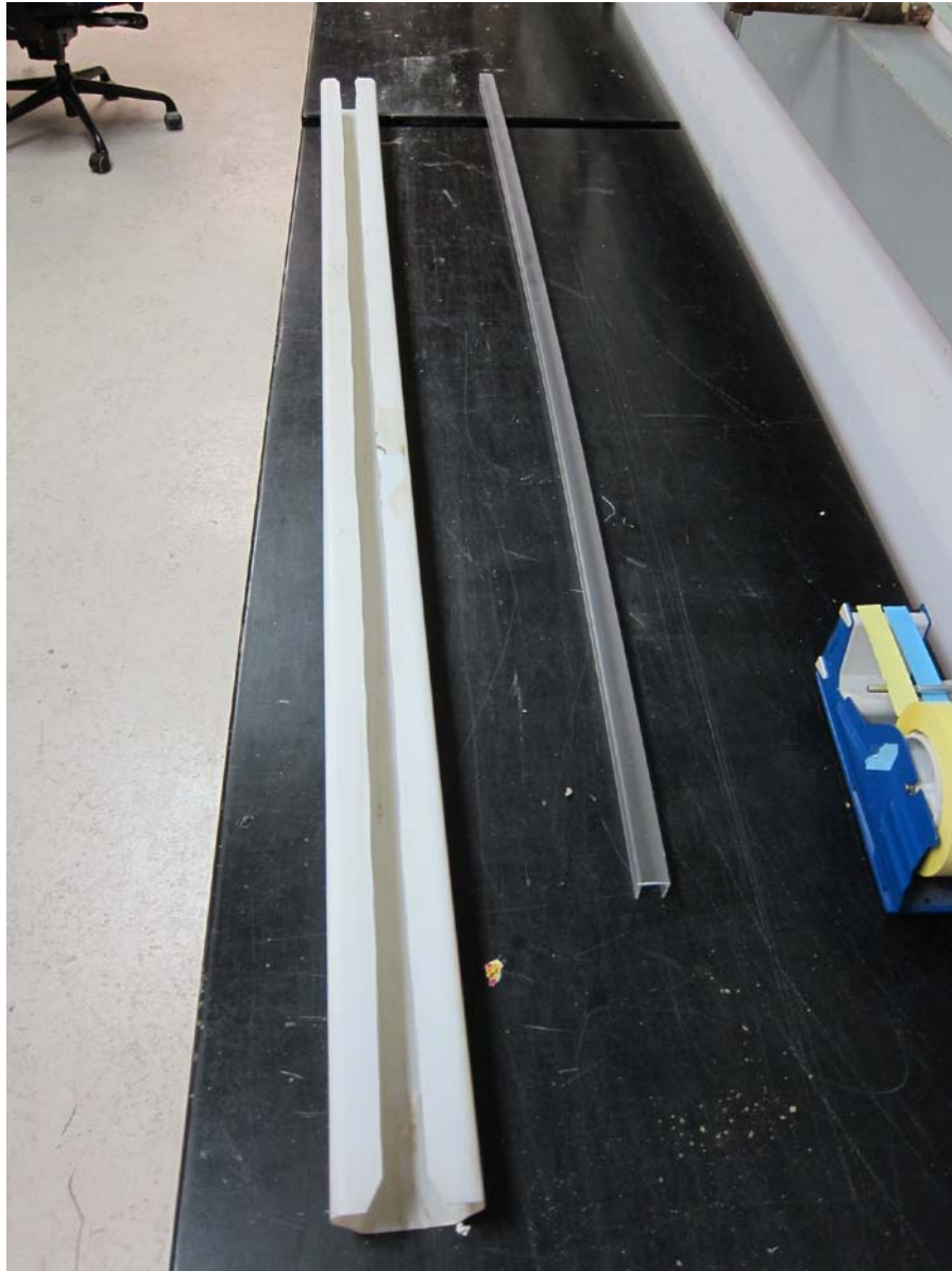
Figure 3. D-tube modified for U-channel sampling of highly unconsolidated sediments.
