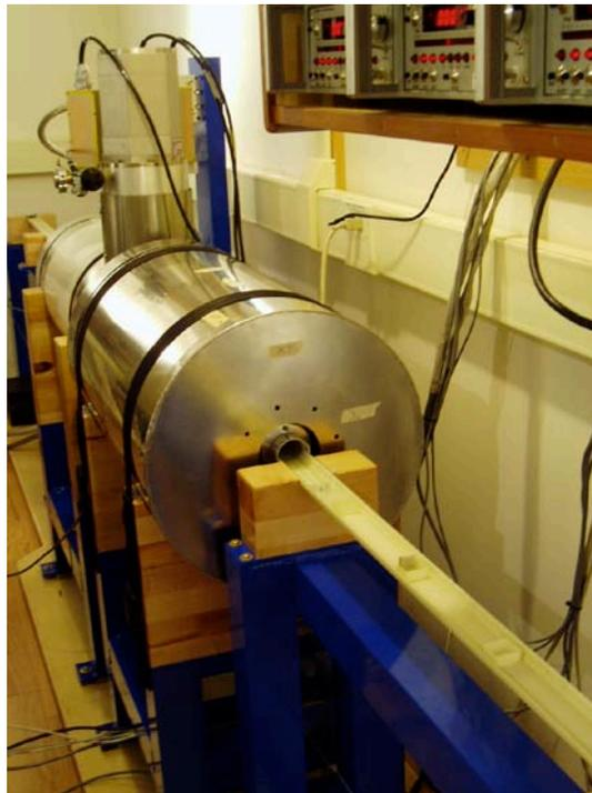
Figure 1. U-channel magnetometer
